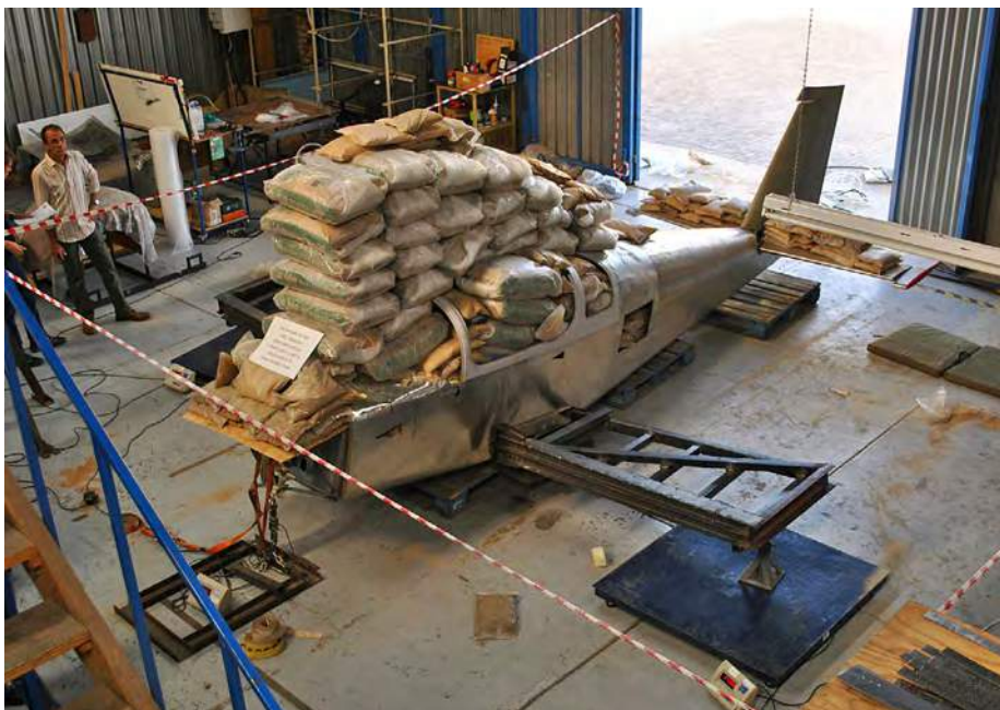
The Airplane Factory's approval submission was first class and included a great deal of evidence of load testing of a sacrificial airframe. Photo: TAF
